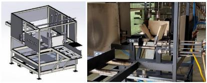
Fig. 2. Charring equipment model and burner setup in real prototype
